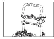
**3** Attach the high pressure hose onto the hose hanger strap.
