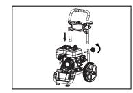
Insert quick-connect nozzles on the bracket of the upper handle unit.
